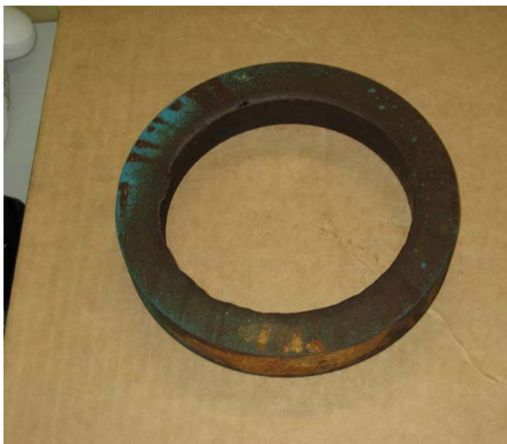
Photograph 4 - Flange on the main structural pin connecting the piling rig to the boom head on the crawler crane
