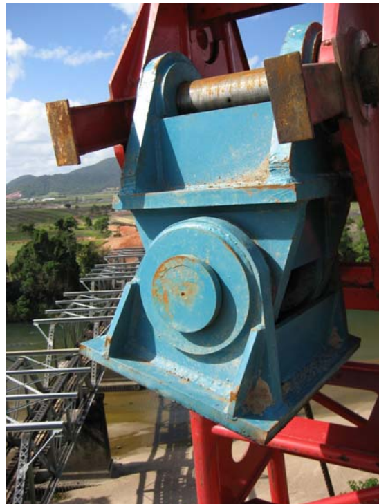
Photograph 2 – Swivel which connects the piling rig tower to the boom head of the crane
